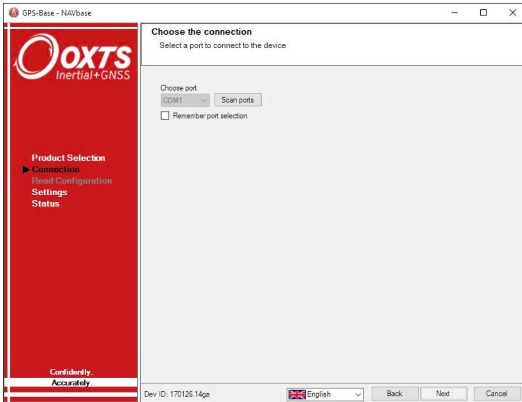
The Connection page is used to specify which port NAVbase should use to communicate with the GPS-Base. If the GPS-Base was not connected when the software was run press the **Scan Ports** button to rescan the ports and find the GPS-Base.
