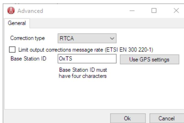
The GPS-Base supports RTCA, RTCA2 and RTCMv3 corrections (RTCMv3 is the default). More detailed information about these formats is available in the section called "Differential correction format details". Is there a differential correction section?
