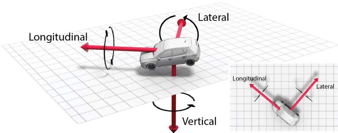
The OxTS horizontal frame is attached to the vehicle. The longitudinal and lateral axes remain parallel to a horizontal plane. The Longitudinal axis is also parallel to the vehicle’s heading when viewed from above.
