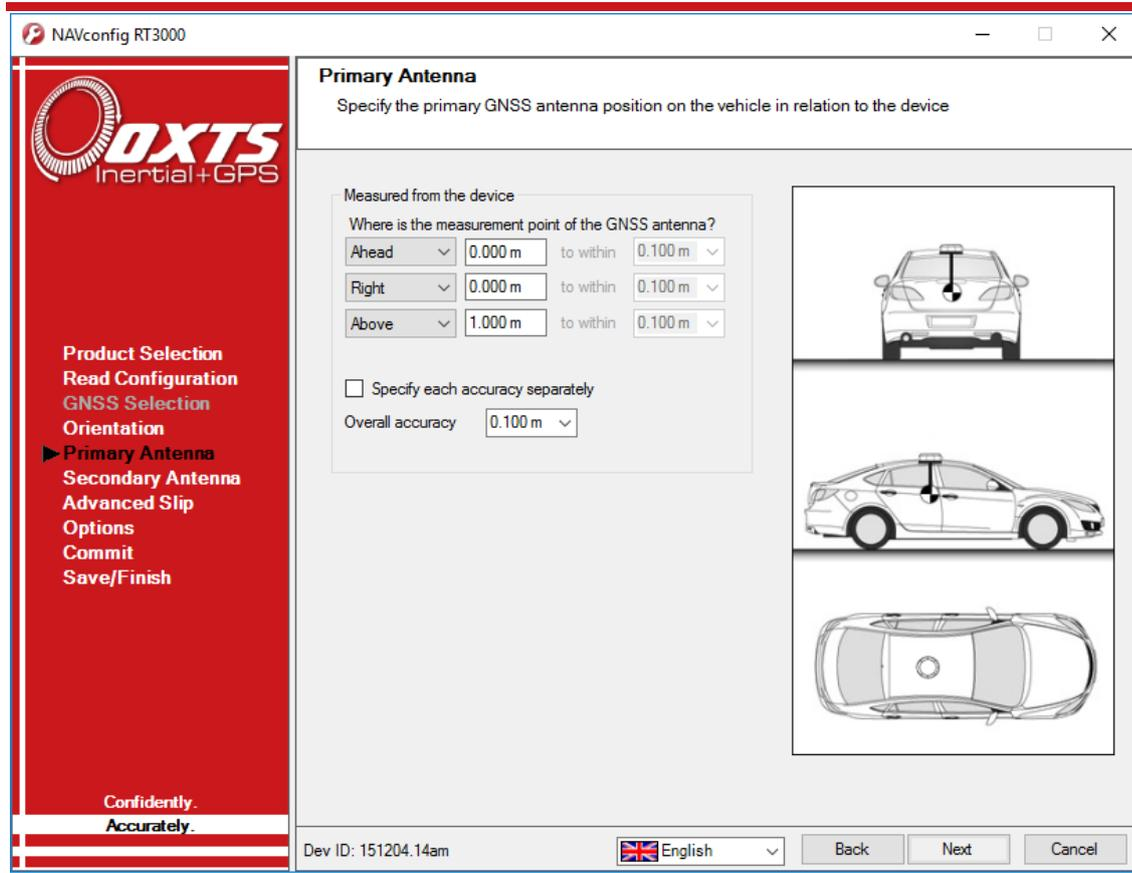
It is necessary to tell the RT the distance between its measurement origin (shown in Figure 6) and the GNSS antenna’s measurement point. This should be entered in the vehicle’s co-ordinate frame.
