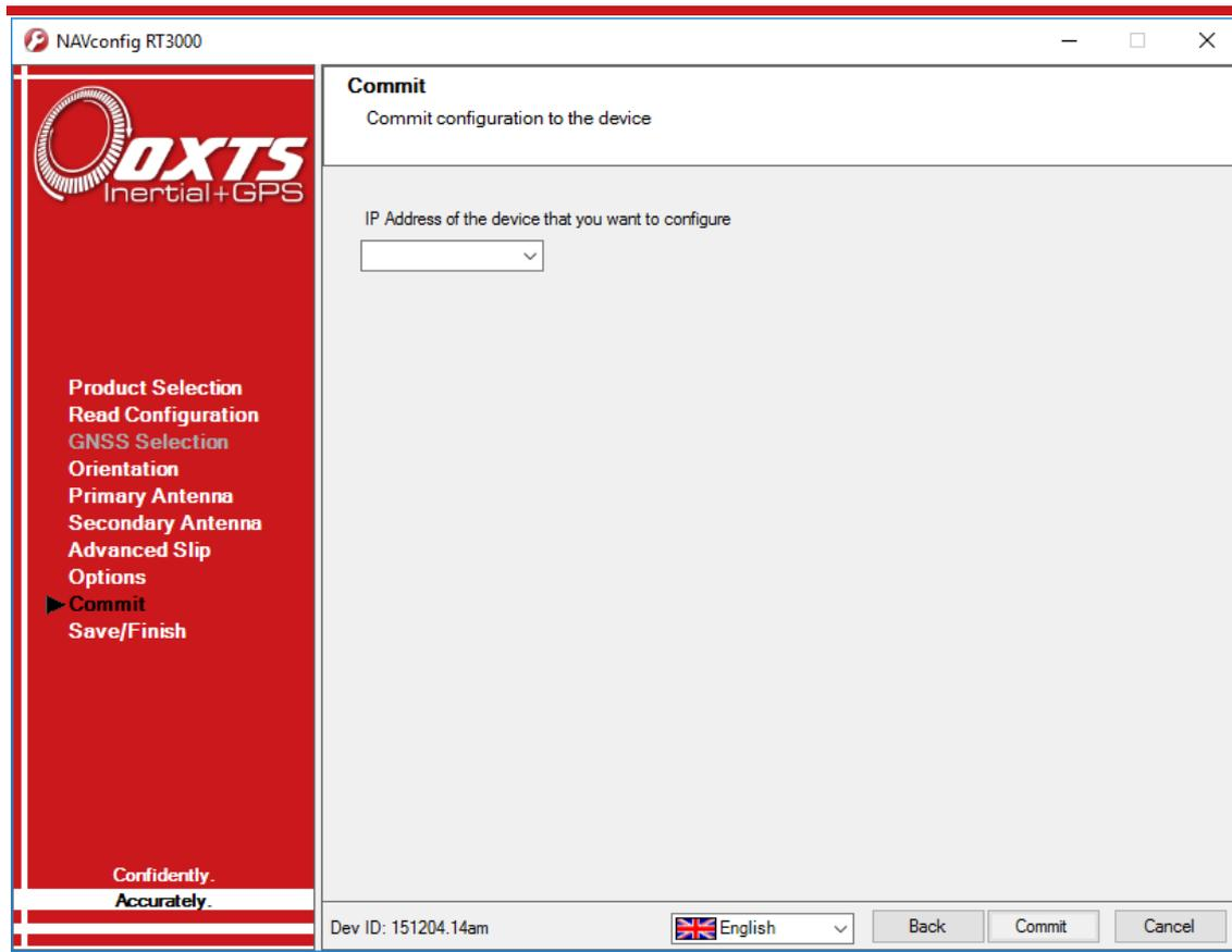
Enter the IP address of the RT you want to configure or select it from the drop-down list. The drop-down box will list all systems currently connected to the computer's network so ensure to select the correct system if there are multiple listed. The list will not function correctly if NAVdisplay or other software is using the RT UDP port unless the OXTS UDP server is running.
