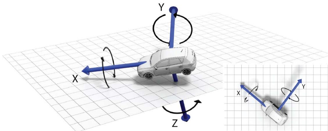
The OxTS vehicle frame is attached to the vehicle and rotates with it in all three axes. The X-axis remains parallel to the vehicle's heading, while the Y-axis points to the right and is perpendicular to the vehicle's vertical plane of symmetry
