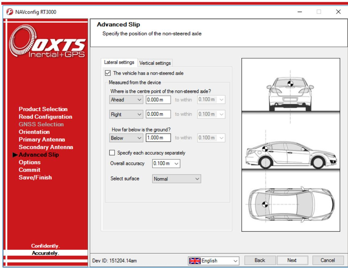
For the **Lateral settings**, the system needs to know the position of the non-steered axle (rear wheels on a front-wheel steering vehicle and vice versa). A position at road height, mid-way between the rear wheels should be used as shown in Figure 26. Vehicles with all wheels steering cannot use this feature reliably, although minor steering of the rear wheels does not significantly affect the results.
