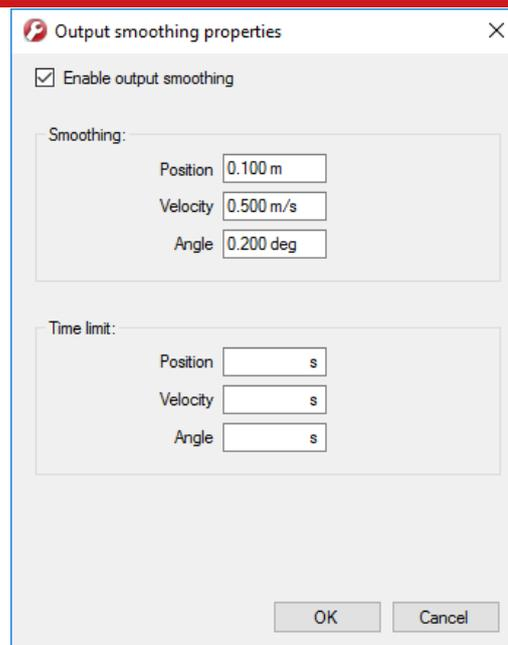
The smoothing of the position, velocity and orientation corrections can be controlled independently. Enter the maximum correction that can be applied every second. For example, if 0.1 m is entered for the position smoothing then the RT will only correct a position error by a maximum rate of 0.1 m/s.
