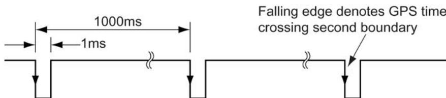
The output is a low-voltage CMOS output, with 0.8 V or less representing a low and 2.4 V or more representing a high. No more than 10 mA should be drawn from this output. Older models have no protection on this output (protection circuitry would disturb the accuracy of the timing). New models (post-September 2013) have limited protection.
