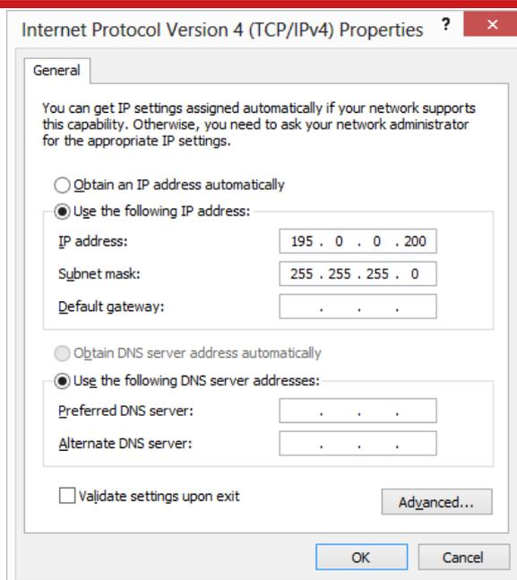
Once the computer is configured the IP address of a RT can be found by running NAVdisplay software; this will display the IP address of any RT connected.
