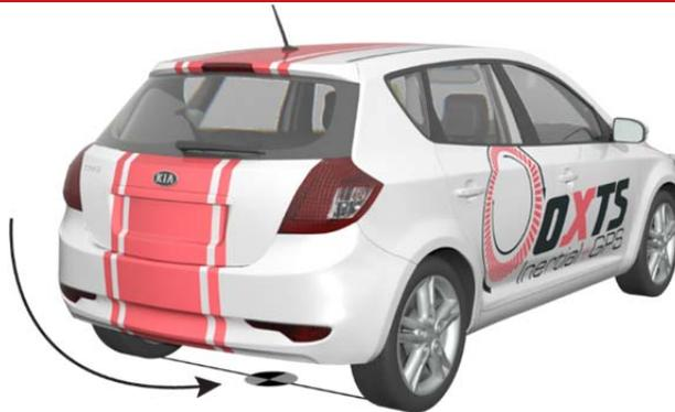
Measuring from the RT, measure the distances to the non-steered axle position in each axis in the vehicle co-ordinate frame. Select the direction from the drop-down lists and enter the distances.
