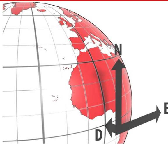
The OxTS navigation frame is attached to the vehicle but does not rotate with it. The Down axis is always aligned to the gravity vector and North always points North.
