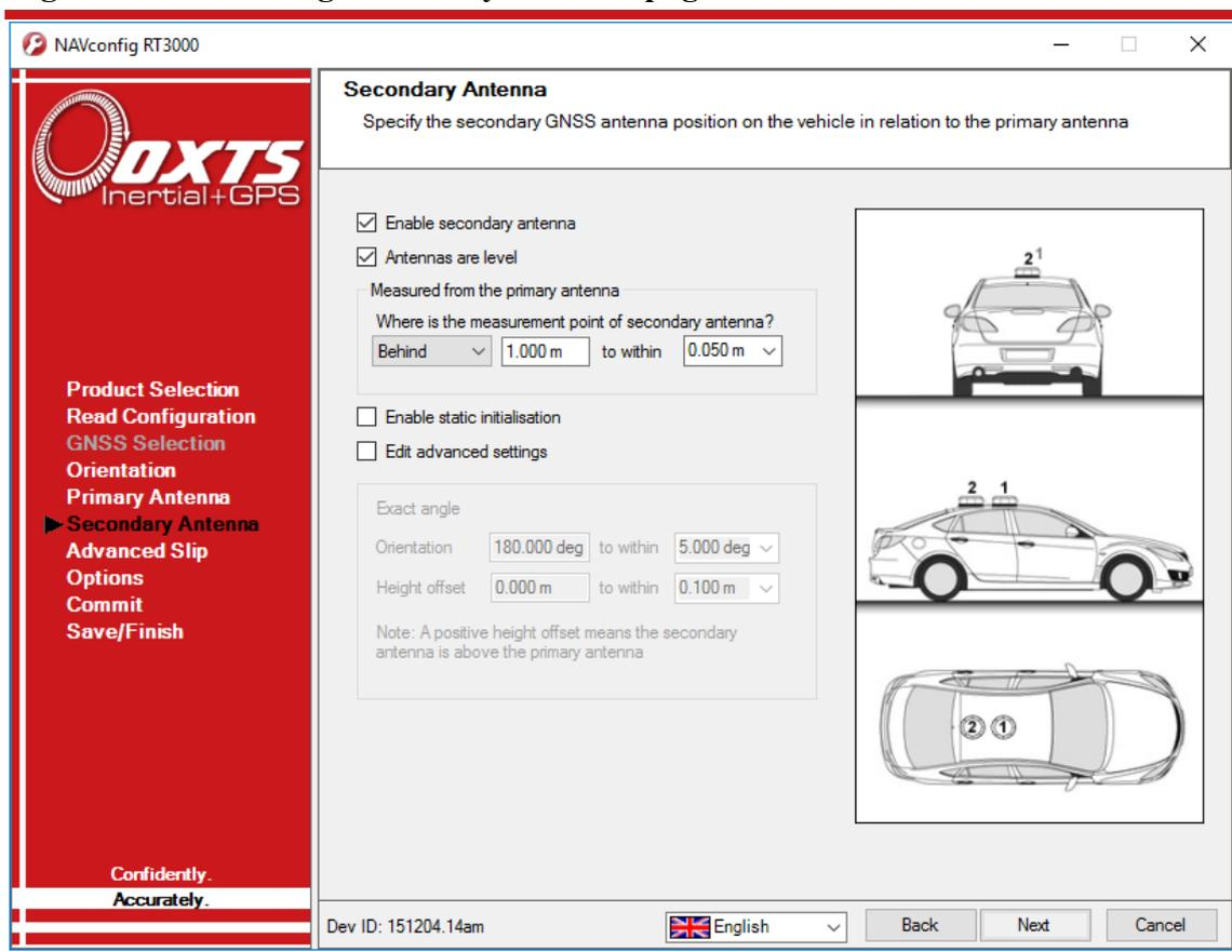
The RT does not estimate the distance between the two antennas. It is essential to get this right yourself, otherwise the system will not work correctly and the performance will be erratic. The measurement needs to be accurate to 5 mm, preferably better than 3 mm.
