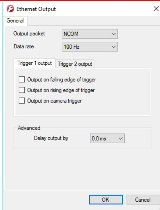
The Ethernet Output can either output NCOM or MCOM, or be disabled by using the **Output Packet** drop-down list. When NCOM or MCOM is selected, the **Data rate** can be selected by using the drop-down list.
