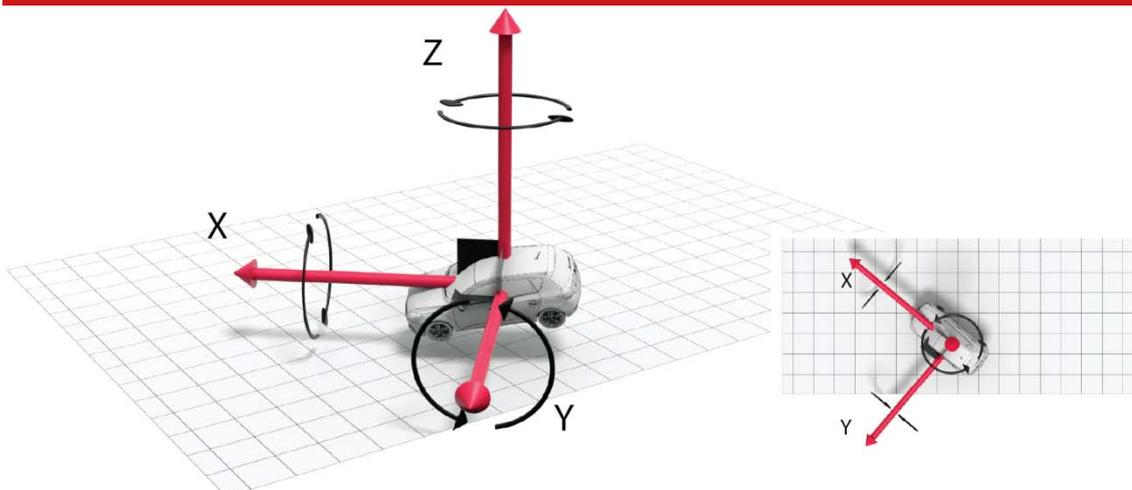
The ISO intermediate system is attached to the vehicle. The X- and Y-axes remain parallel to a horizontal plane. The X-axis is also parallel to the vehicle’s heading when viewed from above.
