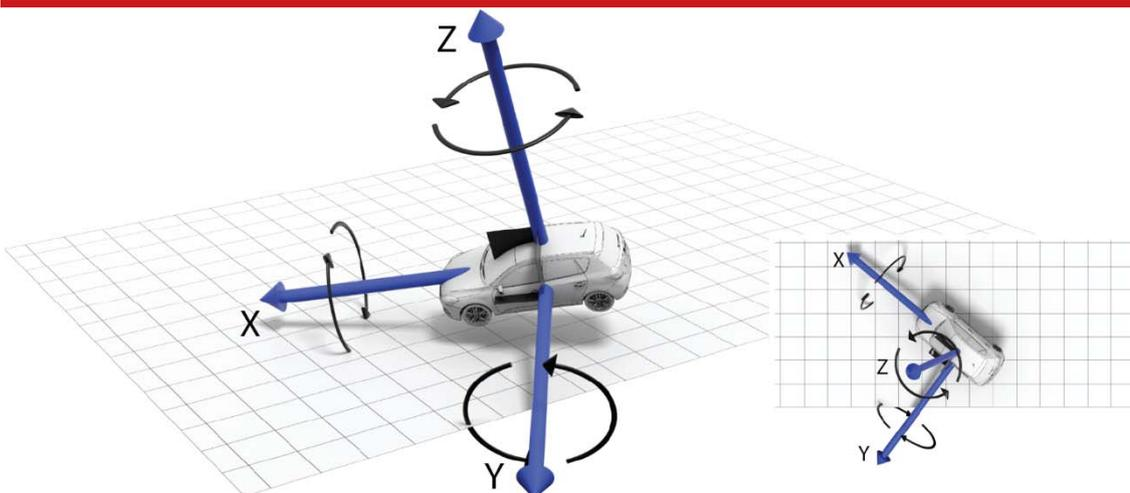
The ISO vehicle frame is attached to the vehicle and rotates with it in all three axes. The X-axis remains parallel to the vehicle's heading, while the Y-axis points to the left and is perpendicular to the vehicle's vertical plane of symmetry.
