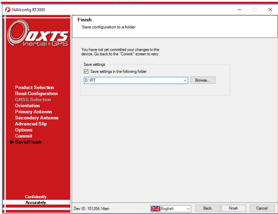
To save a copy of the configuration in a local folder check the **Save settings in the following folder** box and use **Browse...** to select a folder. The configuration has a number of files associated with it so it is recommended to create a new folder. Click **Finish** to save the configuration to the selected folder and close NAVconfig.
