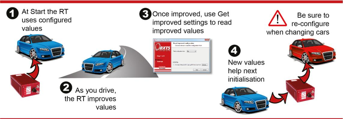
To read the improved values from the RT, click the **Get improved settings** button on the Orientation page. This will open the Get settings from device window, as shown in Figure 21.
