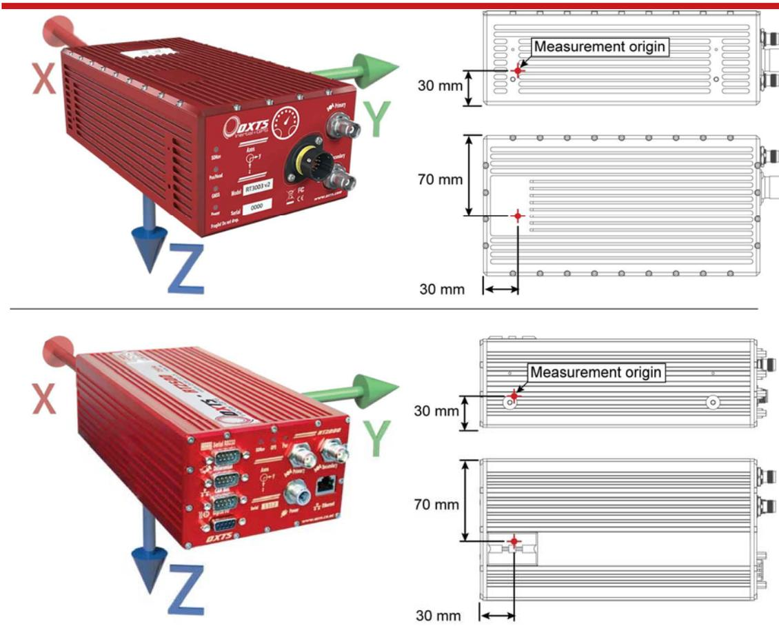
Table 20 lists the directions that the axes should point for zero heading, pitch and roll outputs when the default mounting orientation is used.
