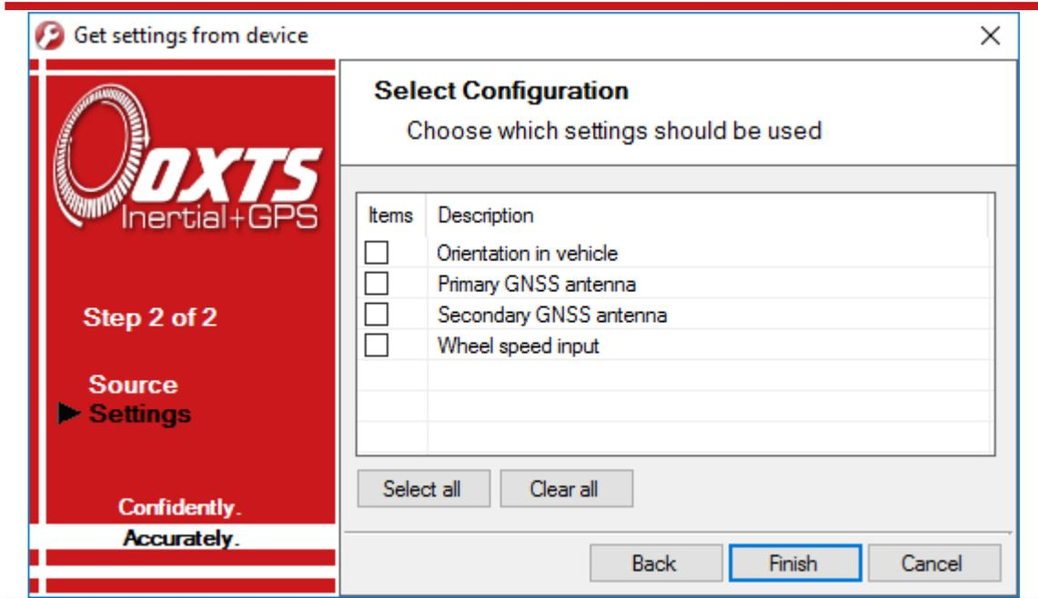
If **Orientation in vehicle** is selected, the improvement to orientation should only be applied if the change in the orientation is small (less than 5°). If the change in orientation is large then it is likely that the original configuration was wrong or has not been loaded into NAVconfig. You are very likely to get poor results if the orientation is changed by a large amount.
