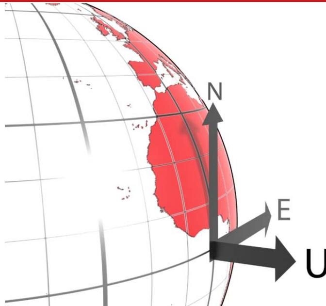
The ISO earth-fixed system is attached to the vehicle but does not rotate with it. The North and East axes are perpendicular to the gravity vector and North always points North.
