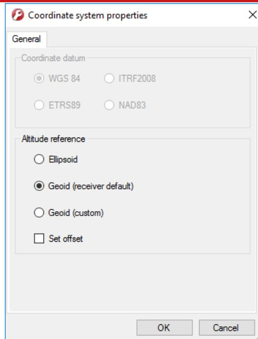
From the **Coordinate datum** section you can choose which reference datum to output latitude and longitude relative to. The default system and the standard for GPS is the WGS 84 datum.
