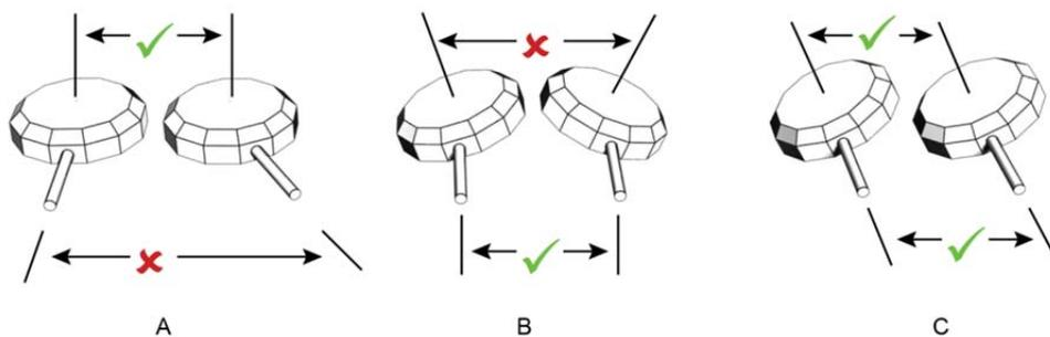
**A)** The bases of the antennas are parallel, but the cables exit in different directions. **B)** The cables exit in the same direction but the bases of the antennas are not parallel. **C)** The bases of the antennas are parallel and the cables exit in the same direction. This configuration will achieve the best results.
