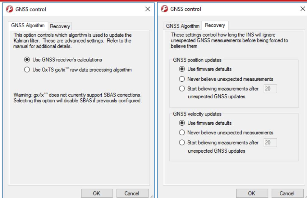
The **GNSS algorithm** tab gives a choice of two algorithms for computing the GNSS measurements. The default option is to use the algorithm provided by the GNSS receiver. Using this algorithm the RT will accept position and velocity from the GNSS and use it to update the Kalman filter.
