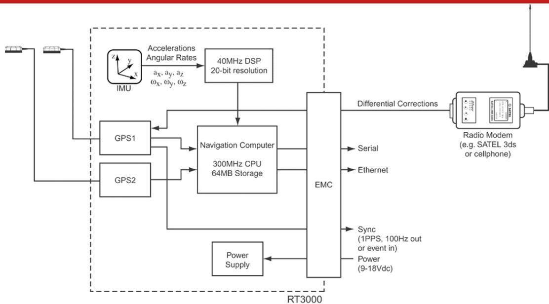
The schematic shows the layout for a dual antenna system, the second GNSS (GNSS2) and the second antenna are not fitted on single antenna systems.
