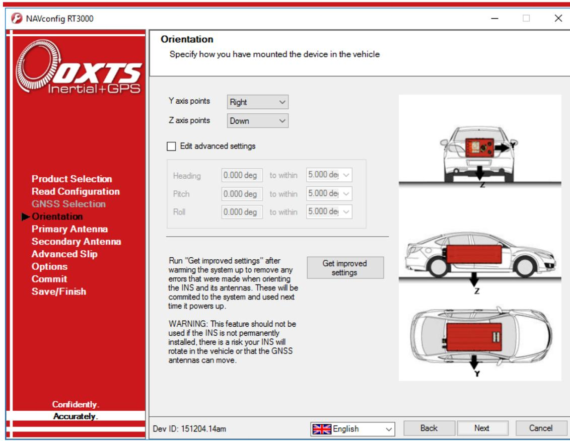
For correct initialisation, it is necessary to get the heading orientation correct. The RT gets its initial heading by assuming the vehicle is travelling forwards in a straight line. If the definition of the vehicle's  $x$ -axis (forward direction) is incorrect in the RT then it will not initialise correctly when the vehicle drives forwards.
