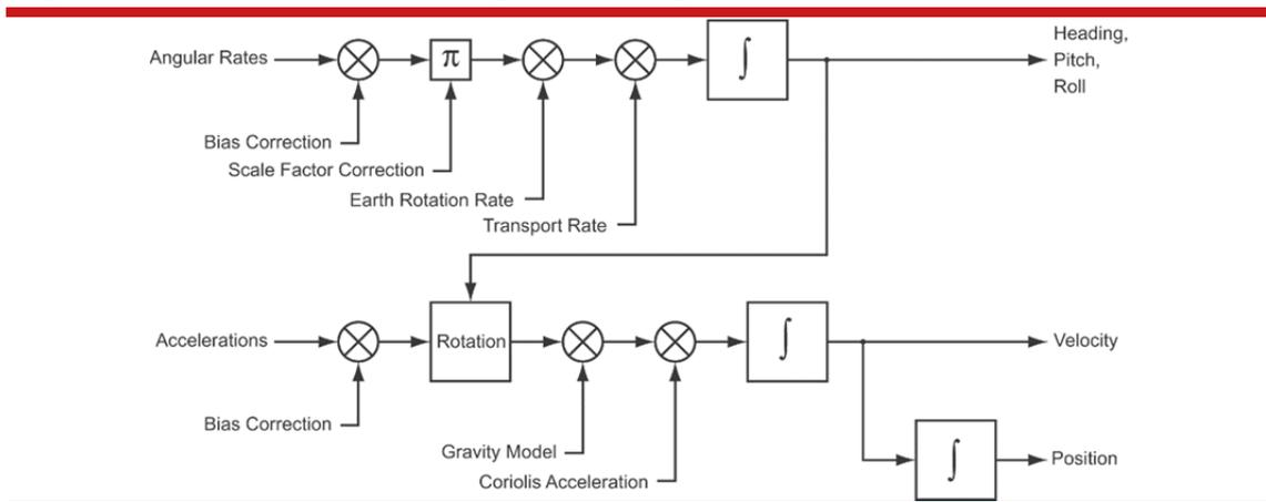
People familiar with inertial navigation systems will note that ‘angular rates’ and ‘accelerations’ are labelled as the inputs. In reality the DSP in the RT converts these to ‘change in angle’ and ‘change in velocity’ to avoid problems of coning and sculling.
