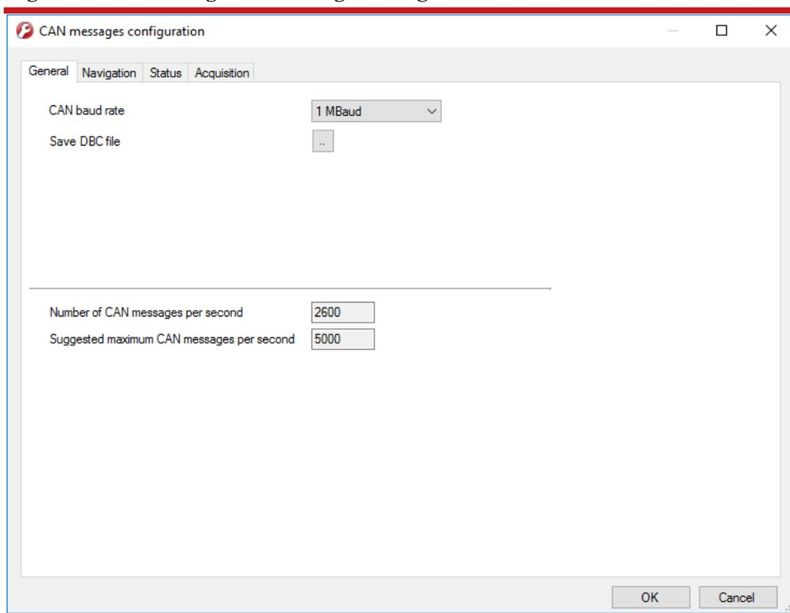
Depending on the baud rate selected, the suggested maximum CAN messages per second will change. A warning message will appear if the combined rate of all current navigation and status messages will overload the CAN bus at the selected baud rate.
