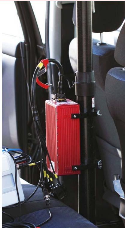
Use the **Y axis points** and the **Z axis points** box to specify which way the RT's axes point in the vehicle. Figure 6 on page 37 shows the RT axes directions. The Orientation page of the configuration wizard, shown in Figure 19, also has illustrations to visualise the orientation of the RT in a vehicle based on the settings input. The advanced settings will change to show the three rotations associated with orientation input even when unavailable.
