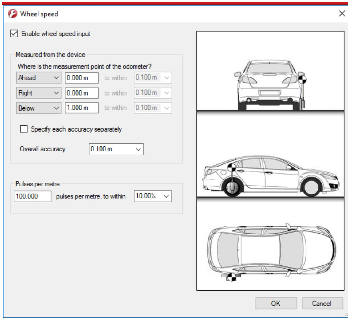
The distances from the measurement point on the RT to the measurement point of the wheel speed encoder in the vehicle coordinate frame should be input. The directions can be selected from the drop-down lists. If the wheel speed is from a prop shaft then the distance should be measured half way between the two wheels. The illustrations in
