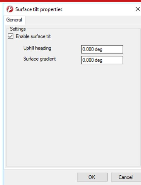
Enter the heading (compared to true north) of the uphill direction and the gradient of the surface.
